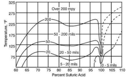
Figure 1 - Steel corrosion rates as a function of sulfuric acid concentration and temperature.
